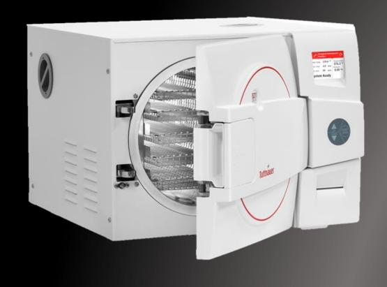
The unit is now ready to run sterilization cycles.
