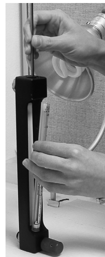
Figure 4-10: Loosen Nut on top of Flowmeter
