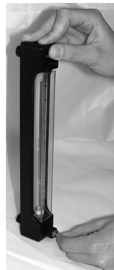
Figure 4-18: Adjust Metal Rod
