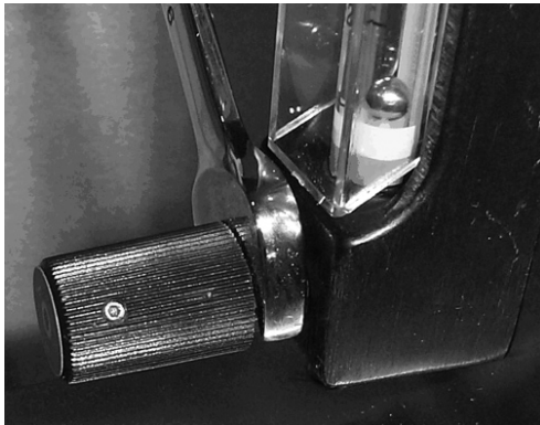
Figure 4-20: Wrench Directly in Front of Plastic Knob
