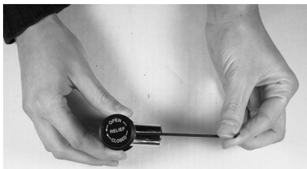
Figure 4-2: Loosen Set Screw on Pop-Off Valve
