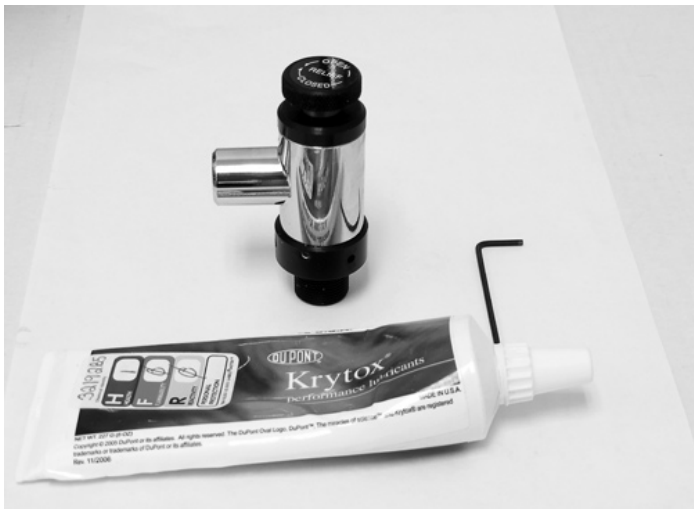
Figure 4-1: Pop-Off Valve Removal (Supplies needed)
