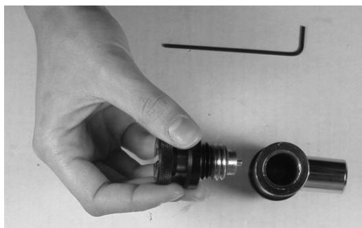
Figure 4-3: Unscrew Assembly from Body
