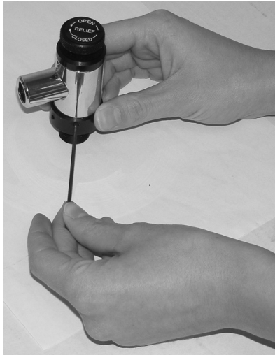
Figure 4-5: Loosen Set Screws
