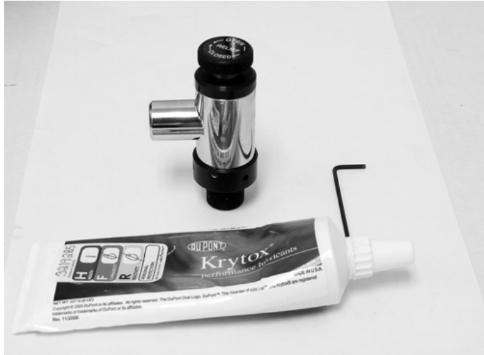
Figure 4-1: Pop-Off Valve Removal (Supplies needed)
