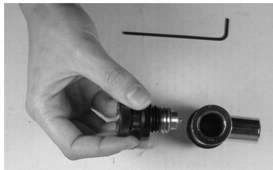
Figure 4-3: Unscrew Assembly from Body
