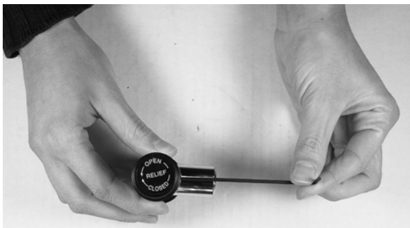
Figure 4-2: Loosen Set Screw on Pop-Off Valve
