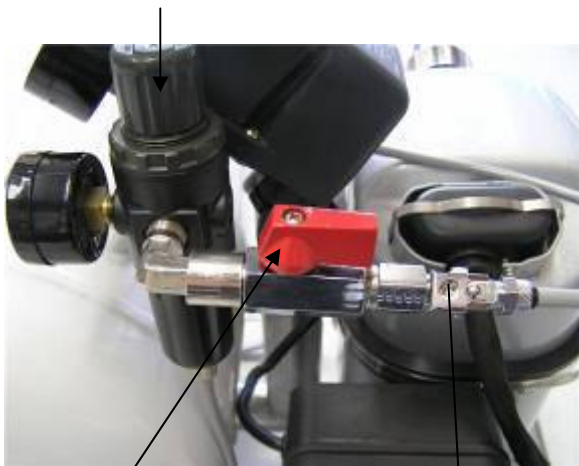
Air ON / OFF (valve pictured in ON or open position)
